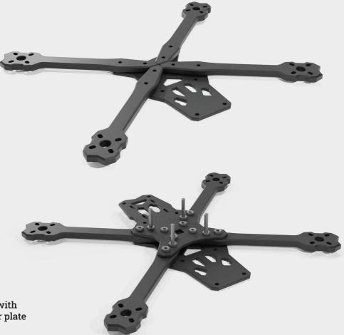
Arms are secured by 8x M3 Cylinder Head screw (2 per arm) with washers against the front plate and pressnuts against the rear plate
